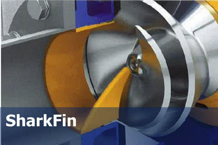
The **SharkFin** is located in the pump suction port and provides an optimized deflection of the incoming solids and fibrous material toward the centre of the impeller. This reduces solids settling and clogging, resulting in significantly less downtime.
